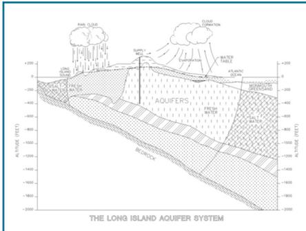
The source of water for the District is groundwater pumped from 23 wells located throughout the community that are drilled into the Glacial and Magothy aquifers beneath Long Island, as shown on the figure above. Generally, the water quality of the aquifer is good to excellent, although there are localized areas of contamination.
