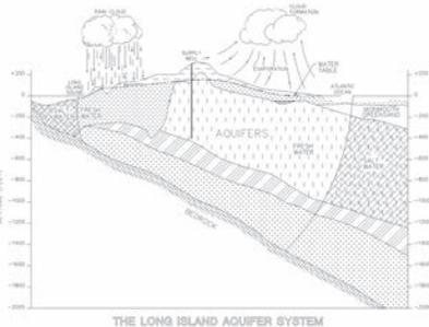
The source of water for the District is groundwater pumped from 18 active wells located throughout the community that are drilled into the Glacial and Magothy aquifers beneath Long Island, as shown on the above figure. Generally, the water quality of the aquifer is good to excellent, although there are localized areas of contamination.
