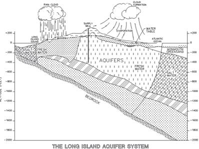
The source of water for the District is groundwater pumped from 18 active wells located throughout the community that are drilled into the Glacial and Magothy aquifers beneath Long Island, as shown in the above figure. Generally, the water quality of the aquifer is good to excellent, although there are localized areas of contamination.
